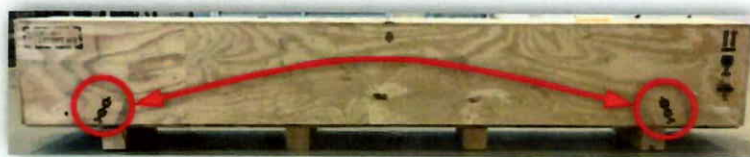
Figure 3.1: lifting points box
