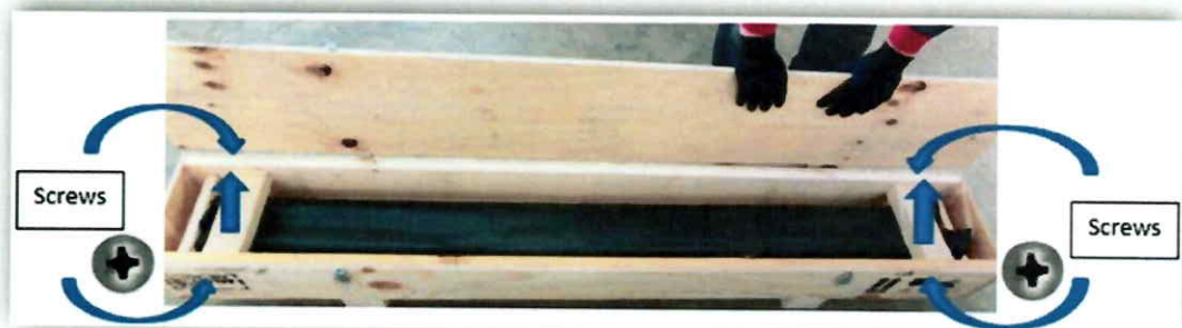
Figure 4.4: remove of wooden beams
