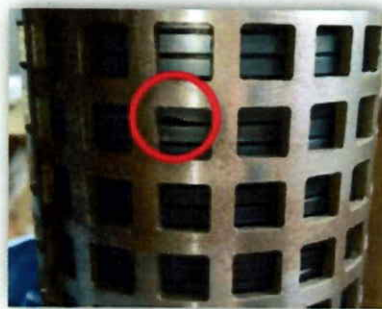
Figure 5.2: not allowed chipping
