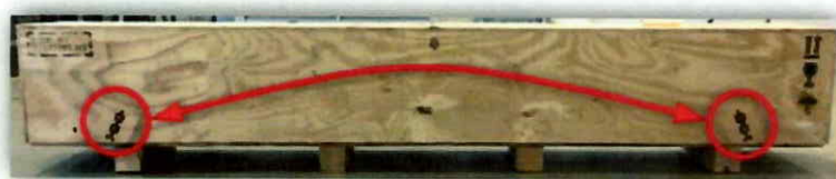
Figure 3.1: lifting points box
