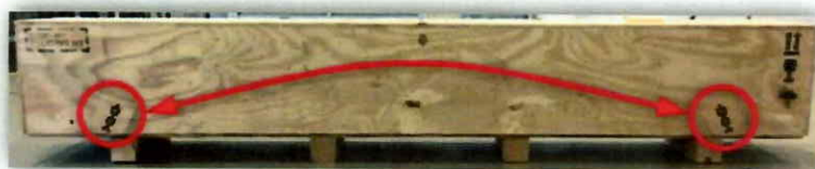
Figure 3.1: lifting points box
